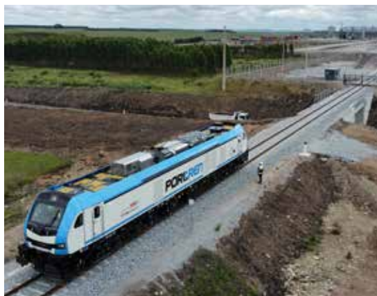
△ The launch of dynamic track testing with a freight locomotive
