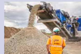
An impact crusher recovers materials for re-use
